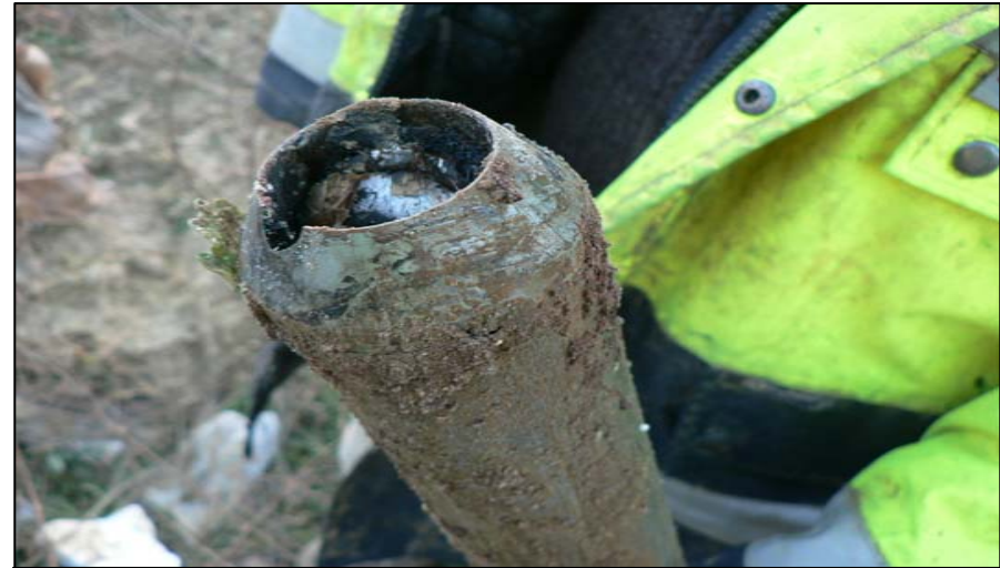
Cutting shoe of damaged Core Sampler with part of protection material of the electric cable
